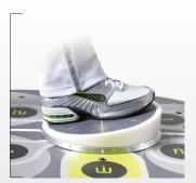
Two foot pads with variable angle of elevation (10° increments) and rotational position (15° increments)
